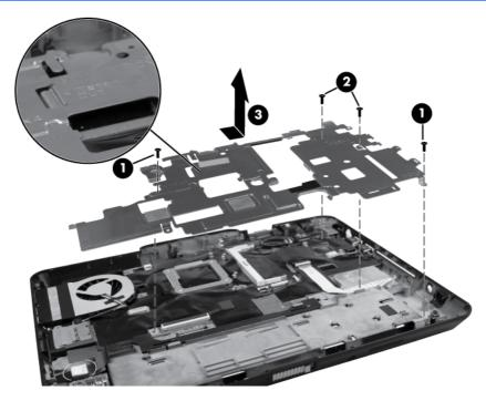
Reverse this procedure to install the system board shield.
